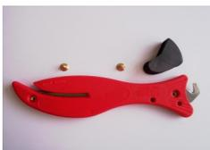
Snap halves firmly back together ensuring there are no gaps. Replace & tighten screws. Replace hook cover
