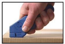
Push down until front face of knife is in full contact against the box. At this point the guards will be fully retracted.
