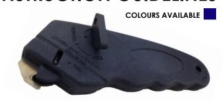
The Boxer 700M is designed primarily for cutting cardboard. It is moulded in a Metal Detectable plastic with a Carbon Steel hook blade, Stainless Steel straight blade and Stainless Steel components. Auto retracting guards sit either side of the straight blade and retract into the knife when in use. Complete with Metal Detectable security key for a controlled blade change and blade storage, inside the knife handle.
